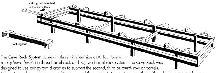
This system utilizes a locking bar (shown above) that connects two sections together without losing any barrel space. The Cave Rack was designed in this fashion so that one person can maneuver a single rack. The rack can be removed easily so the cave floor can be cleaned and the rack does not have any flexion over the span or length of the rack.
